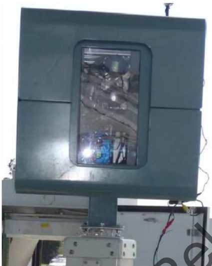
Figure 5 - Cyclops / dtect system in situ during testing on the I-15
