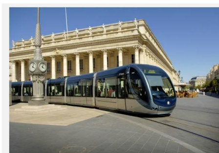
Photograph 8 – Citadis APS in-track power, Bordeaux. (source: Alstom)
