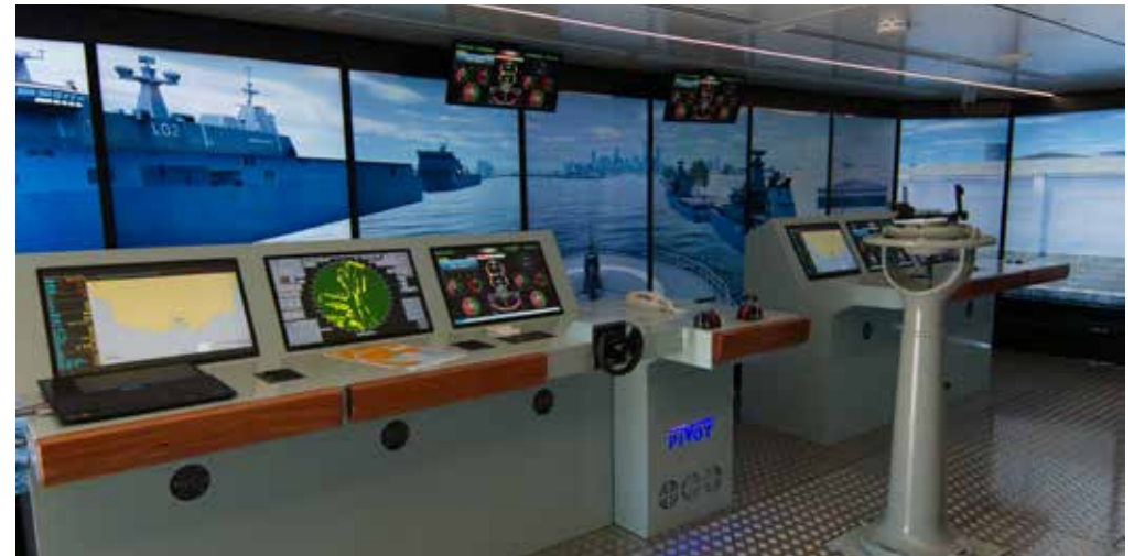
Pivot Maritime International's ContainerSim: Full mission 360° ship's bridge simulator configured in 2x40ft shipping containers.
