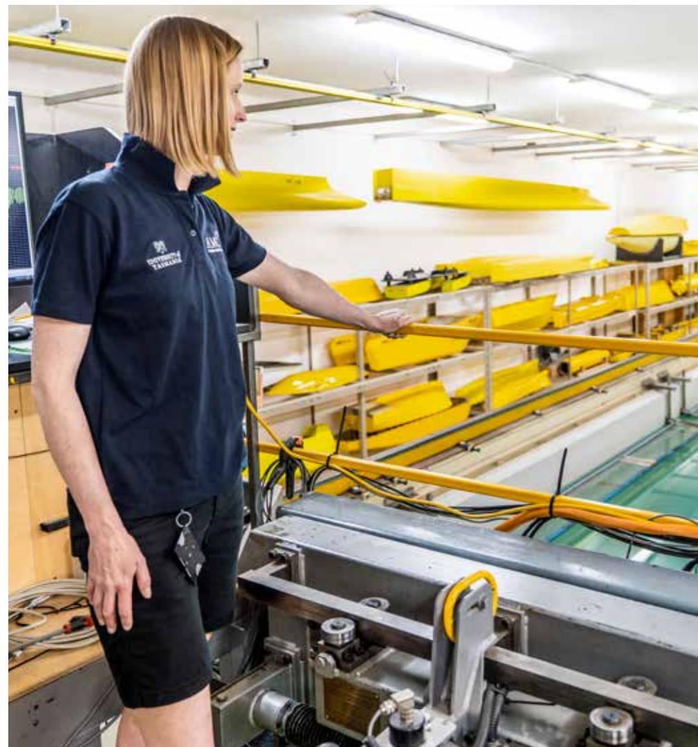
Australian Maritime College's Towing Tank (100 m long by 3.55 m wide), one of two complementary hydrodynamic test basins at the College.
