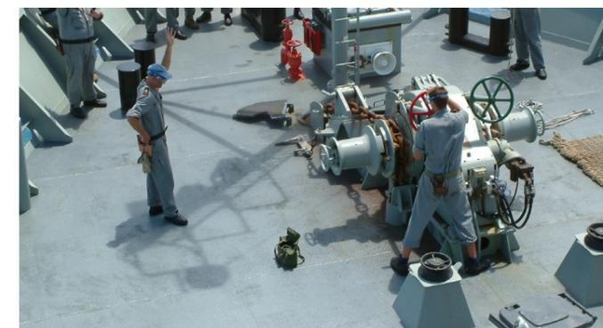
Muir Engineering's Horizontal Windlass HR 22 000 built for high strength 38MM chain on board HMAS *Melville*
