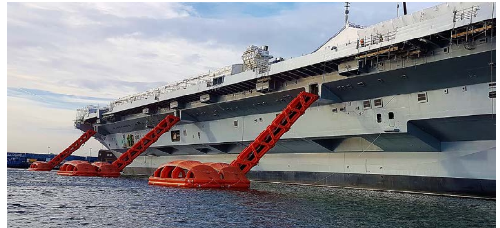
Liferaft Systems Australia Marine Evacuation System installed on the Royal Navy's (UK) Queen Elizabeth class aircraft carriers
