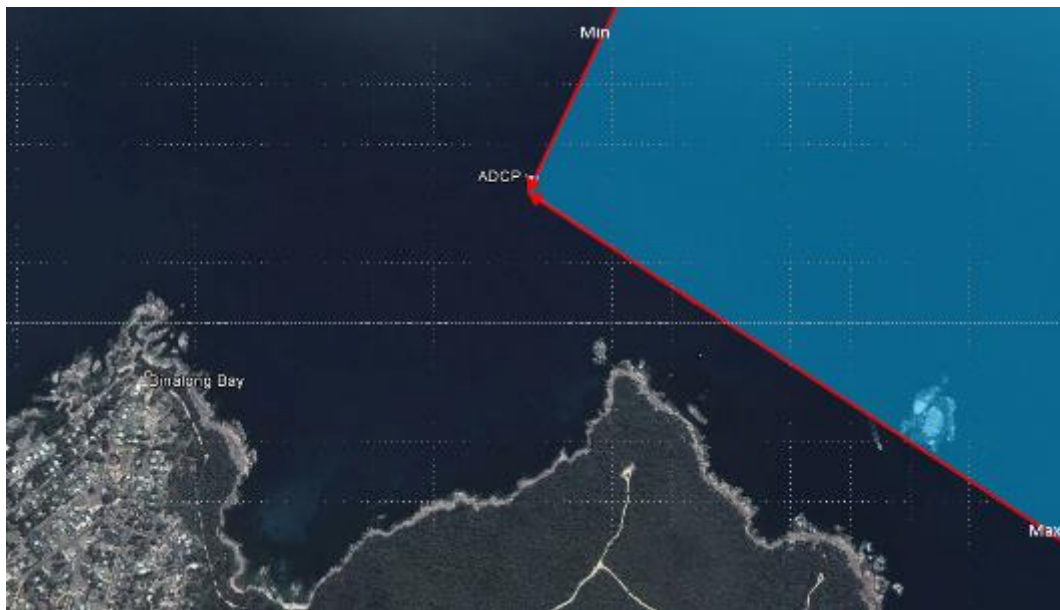
Figure 8 The minimum and maximum average direction (in degrees) of current flow at the proposed scuttling site
