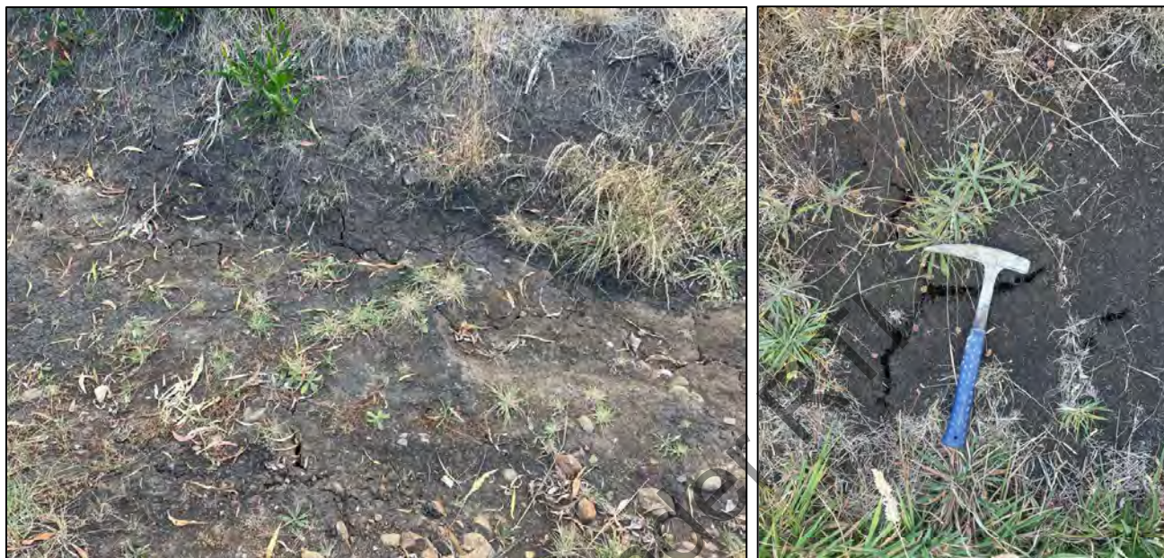
Figure 5 High plasticity surficial soils within the drainage channel (left) and generally across the site (right)
