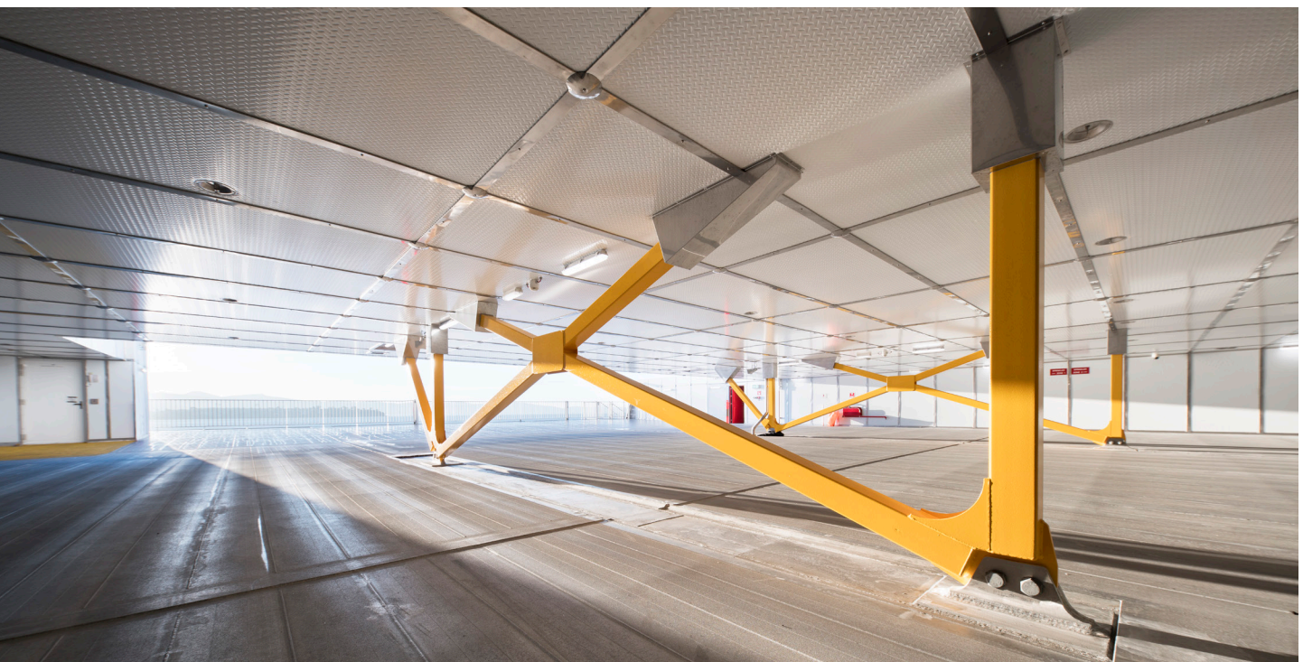
CBG SYSTEMS RAPID ACCESS COMPOSITE (RAC) STRUCTURAL FIRE PROTECTION FORMING THE DECKHEAD AND BULKHEAD OF A HIGH SPEED FERRY
