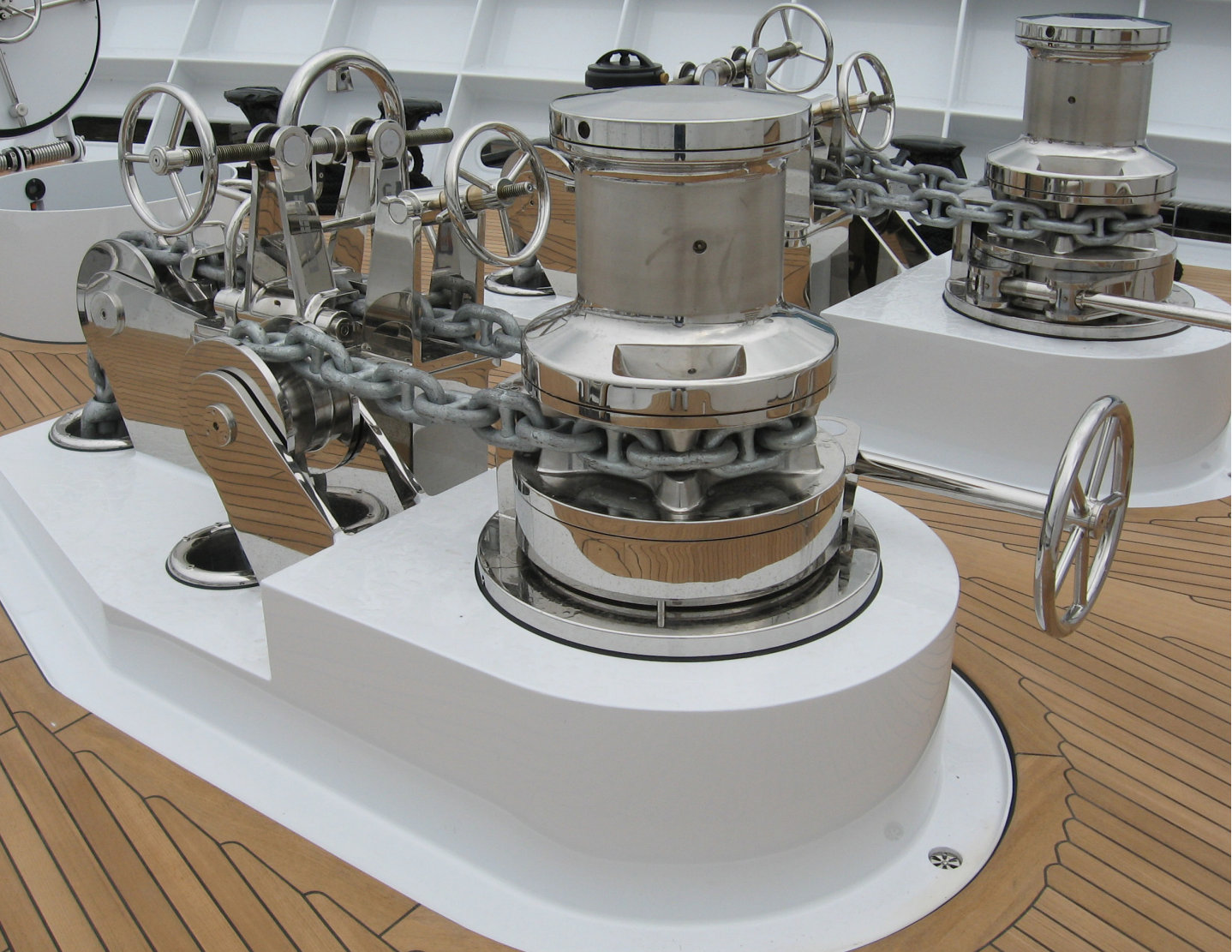
MUIR ENGINEERING ANCHORING SYSTEM COMPRISING VRC 20 000 WINDLASS, RETURN ROLLER ASSEMBLY AND CHAIN COMPRESSOR FITTED TO 65 METRE SUPERYACHT BY FEADSHIP ROYAL VAN LENT
