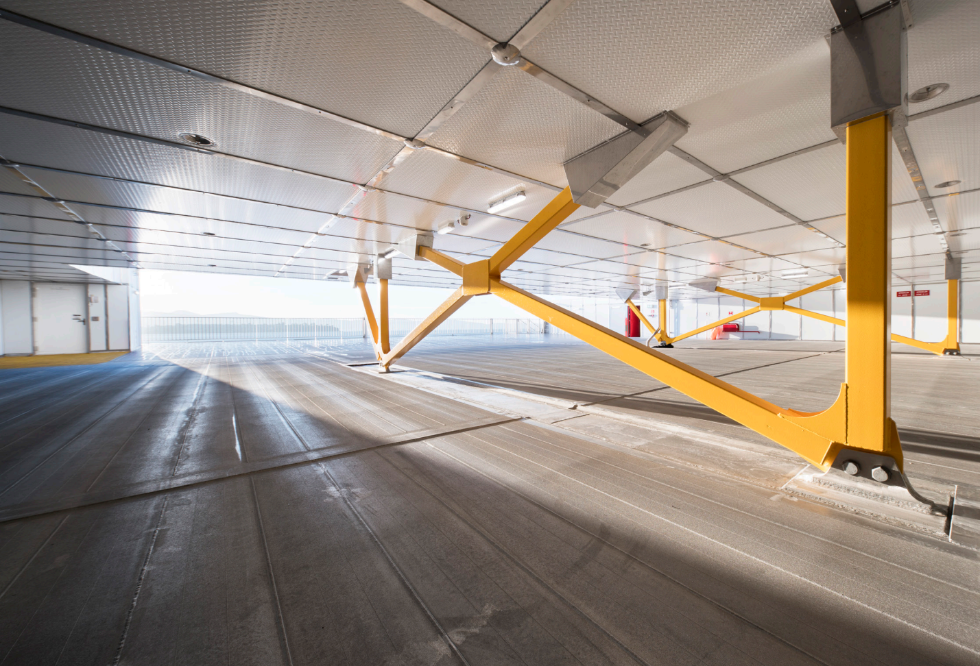
CBG SYSTEMS RAPID ACCESS COMPOSITE (RAC) STRUCTURAL FIRE PROTECTION FORMING THE DECKHEAD AND BULKHEAD OF A HIGH SPEED FERRY
