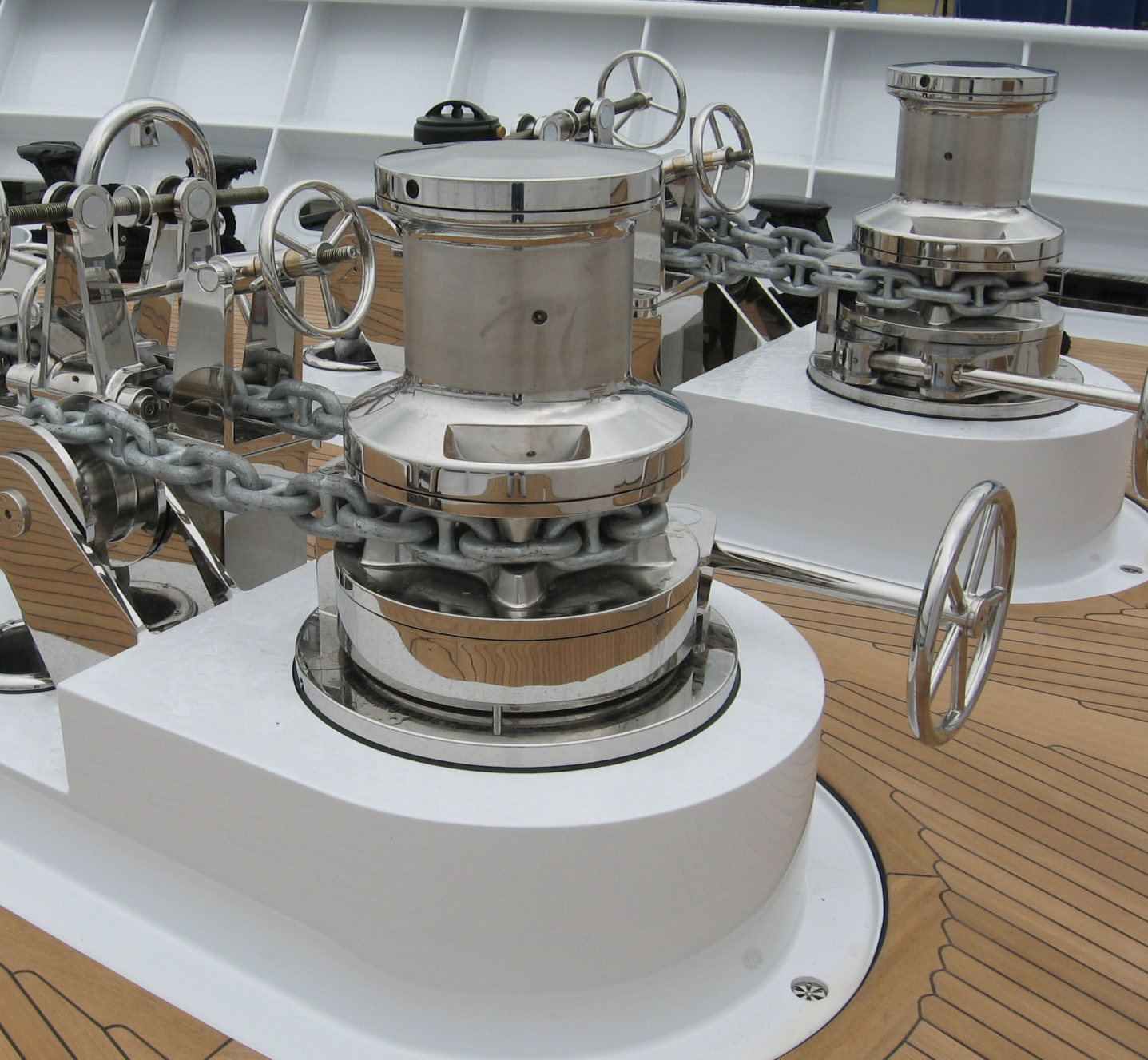
MUIR ENGINEERING ANCHORING SYSTEM COMPRISING VRC 20 000 WINDLASS, RETURN ROLLER ASSEMBLY AND CHAIN COMPRESSOR FITTED TO 65 METRE SUPERYACHT BY FEADSHIP ROYAL VAN LENT
